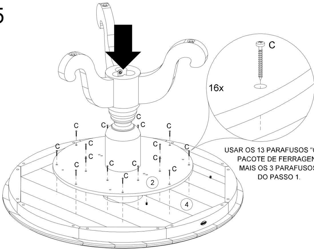
USAR OS 13 PARAFUSOS "C" DO PACOTE DE FERRAGENS MAIS OS 3 PARAFUSOS DO PASSO 1.
